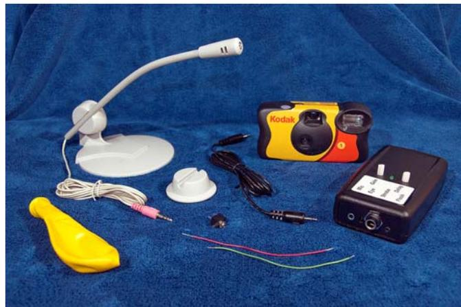
Shown above is a kit from Quaketronics.com. Included is a microphone which is plugged into the black trigger control box on the right. Other miscellaneous parts are used to convert that Kodak camera into an inexpensive remotely triggerable high-speed flash, which is also plugged into the trigger control box.
